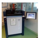
Fluorescence X : measuring wear metals in technicentre
