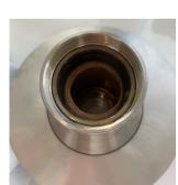
Measuring a grease's dynamic dye penetration (COFRAC)
