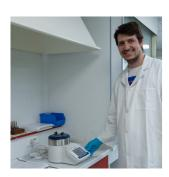
Measuring a grease's dropping point (COFRAC)
