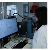
Thermogravimetric Analysis: assessing a grease's lubricating reserve via its loss of mass
