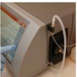
Measuring an oil's viscosity at different temperatures
