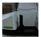
**IR:** identifying a lubricant's footprint / assessing the chemical degradation of a lubricant due to oxidization
