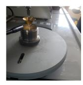
Measuring a grease's worked or non-worked penetrability at ambient or low temperature (COFRAC)
