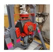
Measuring a grease's resistance to impacts and vibration on the ROPECS and V2F rigs
