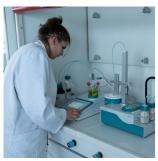
Measuring a grease or oil's moisture content (COFRAC) using a coulometer
