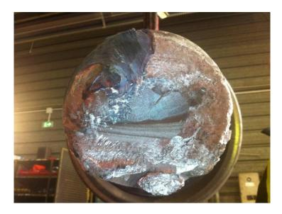
The area where the cracking originated was located. The results were therefore correlated with the maintenance rules and operations to better understand the phenomenon.
